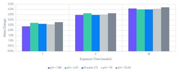
Treatment Method: 5 mm by 5 mm by 5 mm cube submerged in solutions at 40 ° C
