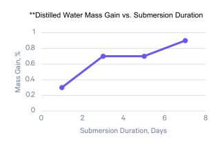
\*Percent weight gained after 1 week submersion following ASTM D543. Values do not represent changes in dimension or mechanical properties.
