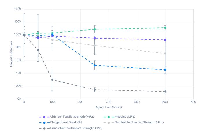
ASTM 4459: Q-Sun XE-1, 0.8 W/m<sup>2</sup>/nm at 420 nm, 55 °C
