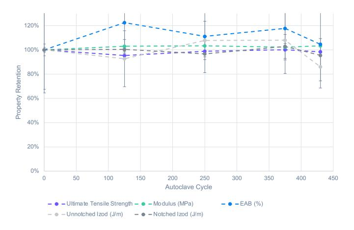
Each cycle consists of a 4 min sterilization at 134°C and 2 min drying time
